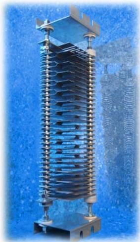
Powerohm offers replacements for roof mounted braking resistors on buses, utilizing punched grid elements for superior cooling over the round edgewound elements furnished by the O.E.M. The flat surface of the grid element allows air to flow over a larger surface area, more effectively cooling the element, reducing fatigue and increasing longevity.
